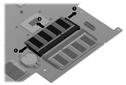
CAUTION: To protect a memory module after removal, place it in an electrostatic-safe container.
